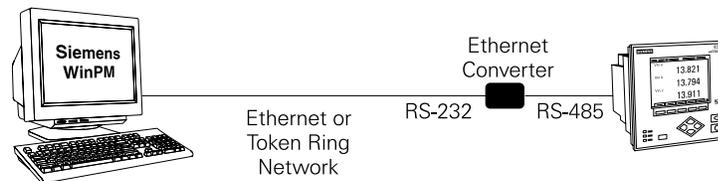
The converter is also capable of connecting up to two protocols, such as SEABus and ModBus RTU.
